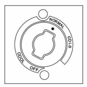
4. The thermostat controls compressor's on/off by sensing inside temperature.
